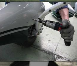
Demount main wheel pants (Philips screw driver)
