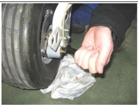
Put an absorbent rag under the wheel brake and use M12 nut wrench to release the hose fiting to the brake cylinder. Do the same on opoosite wheel.
