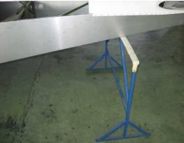
2. Support fuselage aft section as shown on the picture.
