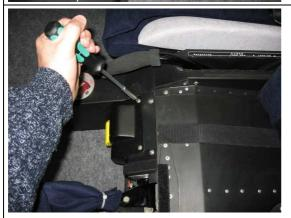
Use Philips screw driver to unscrew parking brake cover attachment screws.
