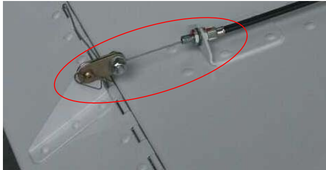
Fig. 1 Trim tab system inspection areas at preflight inspections
