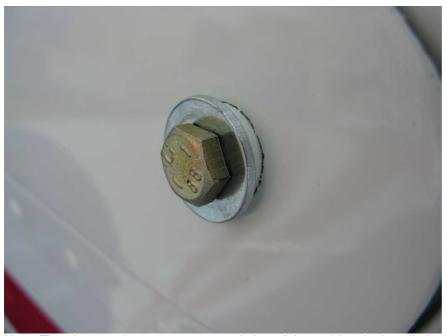
Note. The pictures show a temporary solution of the problem by installation of sutable size washers of approximately 18 mm (3/4") outer diameter and M6 bolts of 30-35 mm length. The washers and bolts sent by the airplane manufacturer may differ.
