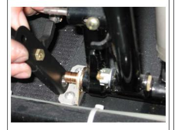
Use nut wrench 9 to screw down nut M6.
