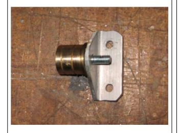
Put the bracket back on its place, set a WASHER 6 on the bolt and screw on nut M6.
