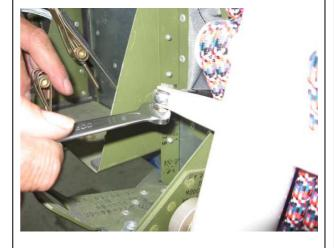
The picture shows 2 washers which adjust clearance of the rod swivel bearing inside the nose leg lever.
