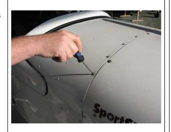
Demount engine upper and lower cowlings to ensure better access to the rods on the nose leg. Use a Phillips screw driver to screw off the cowlings attachment screws. Remove the cowlings
