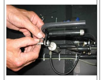
Set the nose wheel as well as the rudder into the neutral position.
