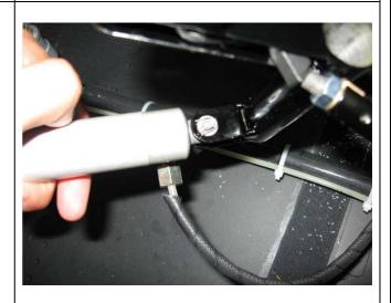
Put the BRAKE PUMP BRACKET E4 90-24 01 back onto the screw.
