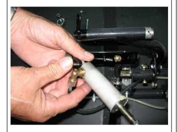
Insert new COTTER PIN 1.6x14 and bent its ends.
