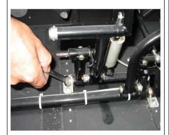
Use Allen wrench 2.8 to unscrew the pedal bottom bracket attachment screws.
