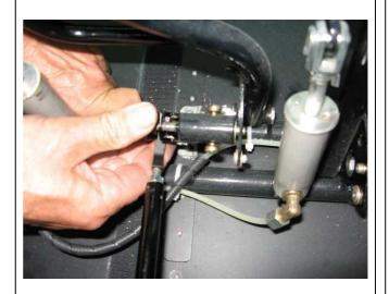
Install new COTTER PIN 1.6x14 to secure the nut.
