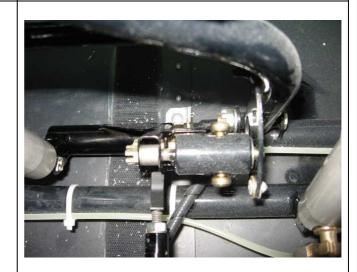
Use a flat screwdriver to screw in the copilot left pedal the small screw.
