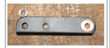
Bent washer tab to secure a nut on the rod end.
