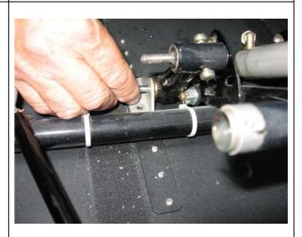
Use Allen wrench 2.8 to screw down the bracket attachment screws.
