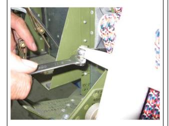
Follow the previous procedure to connect and secure left control rod.
