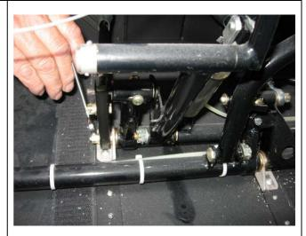
Insert new COTTER PIN 1.6x14 and bent ends to secure it.
