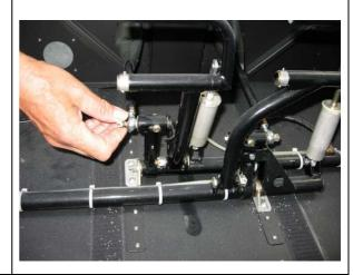
Pull the left rod rear end off the pedal.
