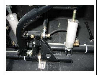
Use the combination pliers to draw out a cotter pin securing the nut of the right rod front end connection bolt to the nose leg lever.
