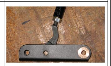
Insert SPACER E4 90-28 01 according to the picture.
