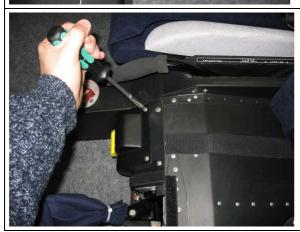
Use a Phillips screwdriver to unscrew the parking brake cover attachment screws.
