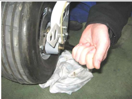
Put an absorbent rag under the wheel brake and use M12 nut wrench to release the hose fitting to the brake cylinder. Do the same on opposite wheel.
