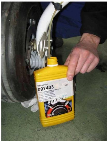
Empty brake fluid into a bottle. Do the same for opposite wheel brake.
