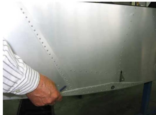
Area of the fuselage reinforcement
