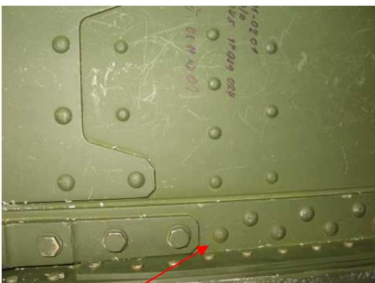
Area of bottom caps with wing-fuselage hinges
