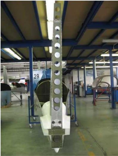
Fin spar with rudder hinges
