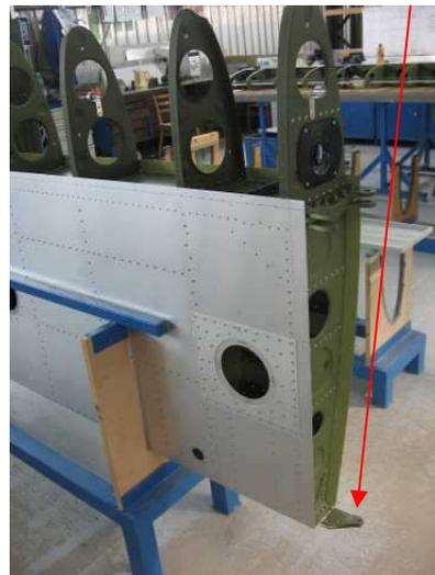
Rear hinge - max.  $\varnothing 8+0.04$  mm
