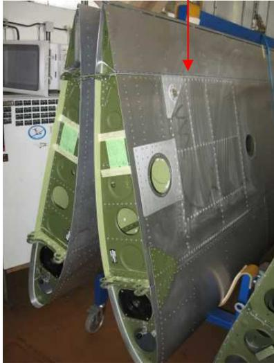
View on the bottom part of the wing in the area of wing-fuselage hinges
