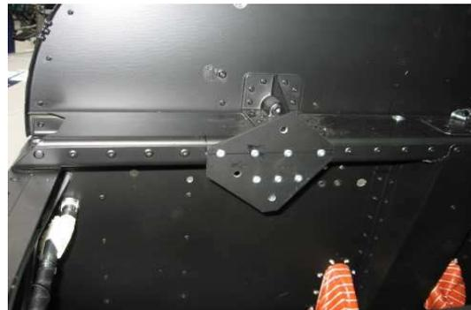
Attachment of the left upper engine hinge on the
