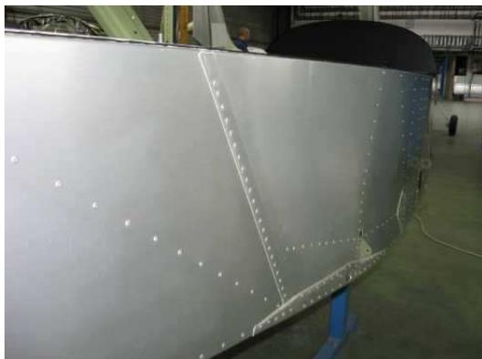
Area of the fuselage reinforcement
