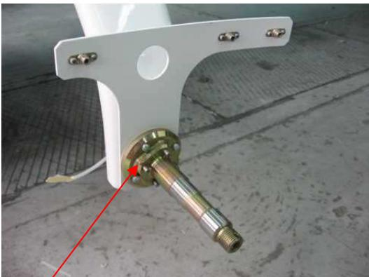
Attachment of the wheel axis with the nose landing gear leg
