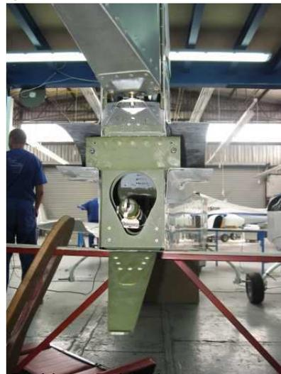
Rudder step bearing
