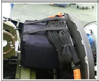
**Note:** For the airplanes with a thermal insulation - put the folded straps on the parachute and fix them to it using a Velcro tape.
