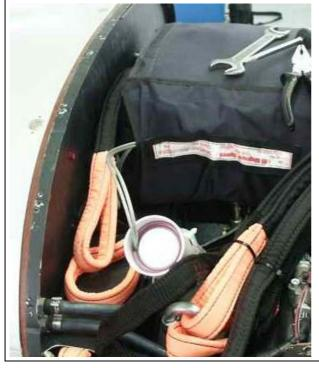
Insert folded part of the right strap between the parachute and firewall and press it down.
