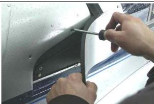
Pull the canopy front side cover away of the fuselage and screw up the screws attaching the cover of a space behind the firewall. Do the same on fuselage opposite side.
