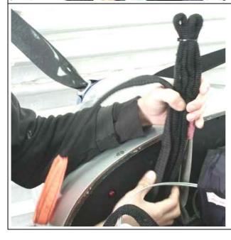
Fold the right strap approximately according to length of the parachute. Leave sufficient length of strap with eye loose to reach the loop eye. Use a tightening strip to fasten folded strap in its upper part.
