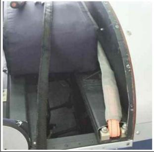
Insert the right strap between the parachute and firewall and press it down.
