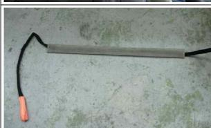
Flatten the wire mesh hose on the strap (e.g. step on it by a shoe). Orient a wire mesh hose bind to be on top when the carrying strap is straightened away of the airplane (see next photo).
