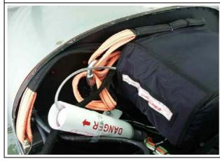
Insert the rear strap between the parachute and firewall, press it down. Insert the left strap on the rear one and press it down.
