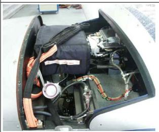
Take out subsequently the carrying straps located between the parachute and firewall and put them on the parachute. Left strap is located upwards.
