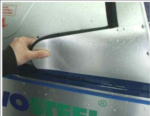
Close the canopy, press slightly the canopy front side cover by thumb to be able to bend it away of the fuselage.
