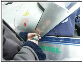
Unscrew the front side screw on both sides of the cockpit canopy.
