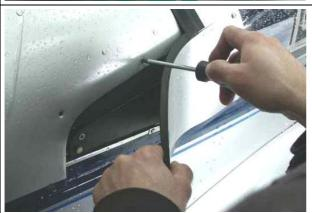
Pull the canopy front side cover away of the fuselage and unscrew the screws attaching a cover of space behind the firewall. Do the same on fuselage opposite side.
