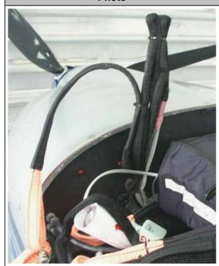
Then use more tightening strips to fasten the folded strap on its bottom and in the middle. Cut overlapping ends of tightening strips.
