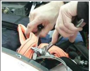
Screw up the loop eye nut and tighten it using M19 nut wrench. Insert a screwdriver into the loop eye to eliminate tightening torque moment.
