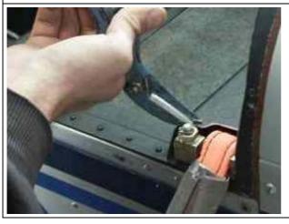
Use right snips to trim upper edge of the channel on the fuselage right side in place of the strap attachment.
