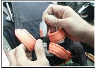
Unscrew the loop eye nut and remove the right strap.
