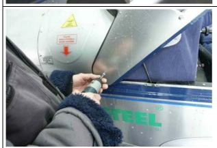
Screw up front side screw on both sides of the cockpit canopy.
