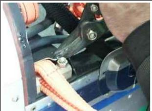
Use left snips to trim upper edge of the channel on the fuselage left side in place of the strap attachment.
