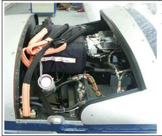
The rear strap is located under the left strap and the right one is on bottom. Take out these straps and put them on the parachute.
