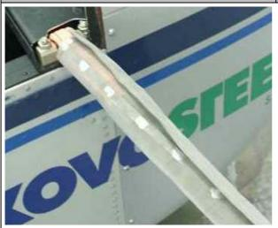
Complete folding along the entire length of the hose up to the strap attachment point to the airframe.
