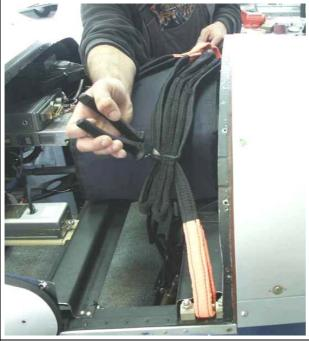
Cut tightening strips of the right strap. Strips hold strap in folded state.
