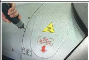
Tighten upper cover attachment screws.
