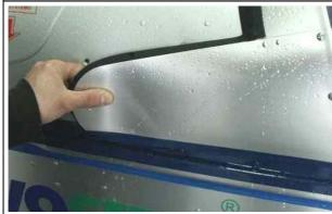
Close the canopy, press slightly the canopy front side cover by thumb to be able to bend it away of the fuselage.
