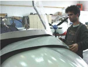
Partly open the canopy and re-install upper cover of the space behind the firewall.
