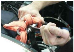
Use M19 nut wrench to loose a nut of loop eye connecting the straps. Insert a screwdriver into the loop eye to eliminate releasing torque moment.
