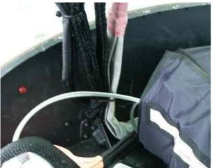
Fold the strap with the wire mesh hose back in point where is the parachute end. Bending radius must not be acute, fold the hose for example over a finger.
