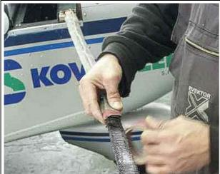
Use a fabric (carpet) tape to wrap shown end of the wire mesh hose with the strap.
