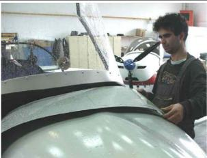
Tilt slightly the canopy from fully opened position and remove upper cover.
