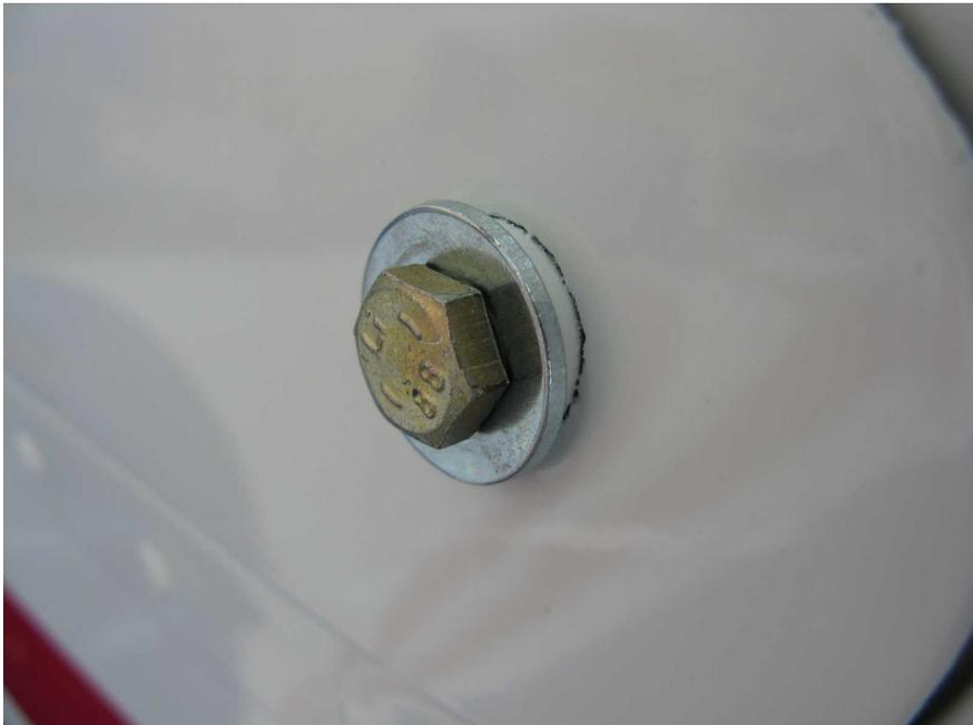
Note. The pictures show a temporary solution of the problem by installation of suitable size washers of approximately 18 mm (3/4") outer diameter and M6 bolts of 30-35 mm length. The washers and bolts sent by the airplane manufacturer may differ.
